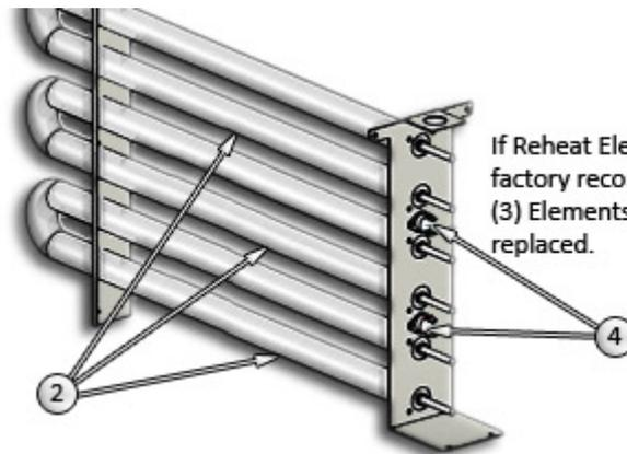
If Reheat Element has failed, the factory recommends that all (3) Elements and the GCD be replaced.
