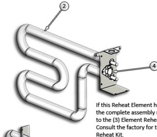
If this Reheat Element has failed, then the complete assembly must be changed to the (3) Element Reheat Assembly. Consult the factory for the replacement Reheat Kit.
